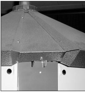
**P 10.** Place 5/16 star washer [Y] over threaded stud above pulley, then add perch assembly [11]. Fasten in place using 10-24 keps nut [B]. (Refer to exploded view on page 6.)
