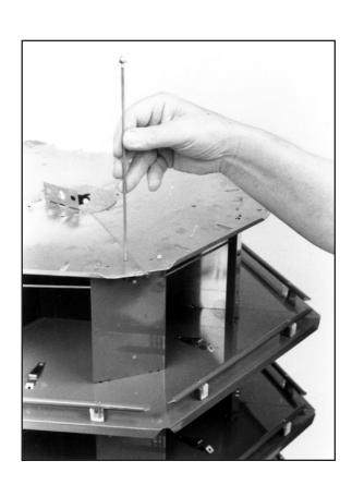
**8.** Turn house on side and inspect round end tabs and door rods for correct location. Readjust if required.
