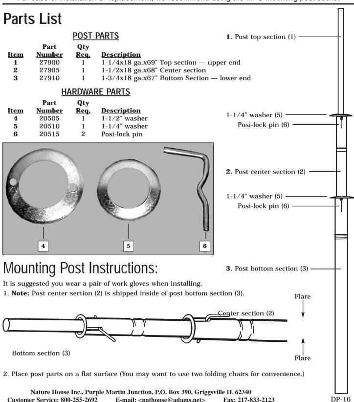
3. Bottom end of top section (1) and center section (2) are flared. When assembled, this flare acts as a stop to prevent raising a section too far. To assemble, it is necessary to slide smaller section through the next larger section from bottom end.
