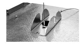
**11.** Insert loop of cable through hole in center of roof (3) and allow roof to settle onto ceiling with ceiling flanges inside roof assembly. Fasten roof to ceiling with six 6x3/8 sheet metal screws (34). Do not over-tighten.
