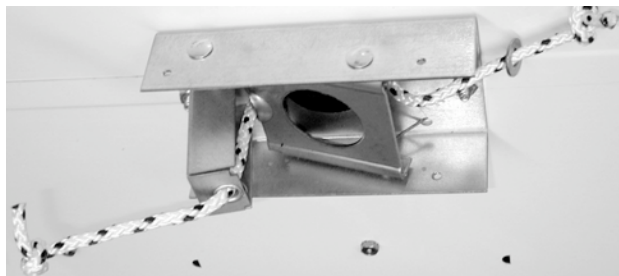
Underside view of floor /lanyard lock assembly
