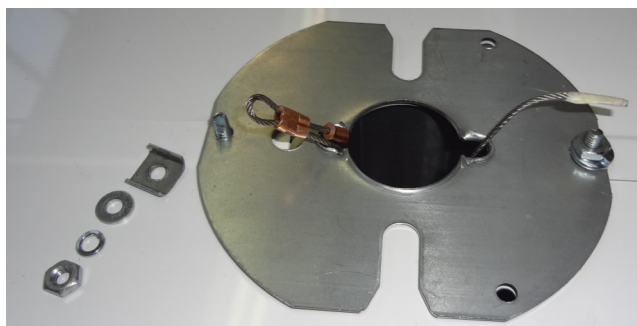
Bottom plate shown attached to the bottom of the house with cable and components
